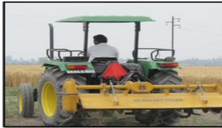
Treatment T 3 - Rotavator (200 cm wide with 8 flanges, 3 flanges in use while others removed)
