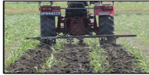
Treatment T 2 - Cultivator 11 tine (6 tines in use and others removed)
